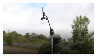
With the aeroclimatic station it is possible to measure temperature, wind direction and precipitation.
